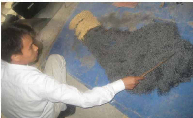
Figure 3: Char and remain rice husk separation
