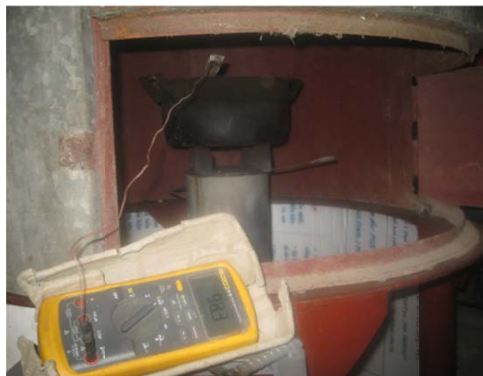
Figure 2a: Above: The stove testing system at Stove Testing laboratory, LHERE. Below: a side view of a stove (the Viet stove) on the testing platform, with the front door of the exhaust hood open to view the set -up.
